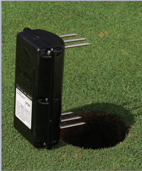
Wireless Sensor Measures Moisture, Temperature and Salinity Levels
